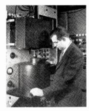
COLOR SLIDE television camera developed by RCA for its all-electronic color television system is being inspected by Ray D. Kell, head of television research section of RCA labs. Light beams from the kinescope are focussed through the slide and separated into component colors by mirrors, which pass the rays to photoelectric cells.
