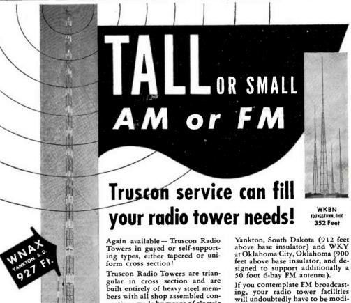
gular in cross section and are built entirely of heavy steel members with all shop assembled connections made by means of electric arc-welding.
