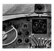
Instrument Panel of the Future. The Teleran indicator, mounted in a cockpit, greatly simplifies the pilot's job with its quickly understood picture showing his position relative to the airport and to other planes in the vicinity. It promises to become one of the most useful developments in the history of aviation.
